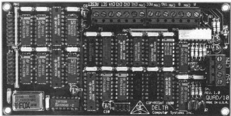
The QUAD/10 module electronically converts quadrature encoder phase signals to equivalent Temposonics® linear transducer signals. Specific applications of the module vary widely, however the QUAD/10 module is particularly useful when an application using a multi axis controller (ie, DELTA's VMC 186/40, MC 186/40 and TMC 188/40 modules) needs to work with a rotary encoder.
