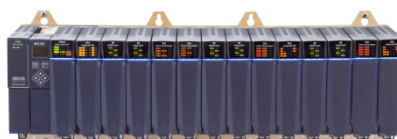
RMC200 on B15 Base Module (up to 32 axes)
